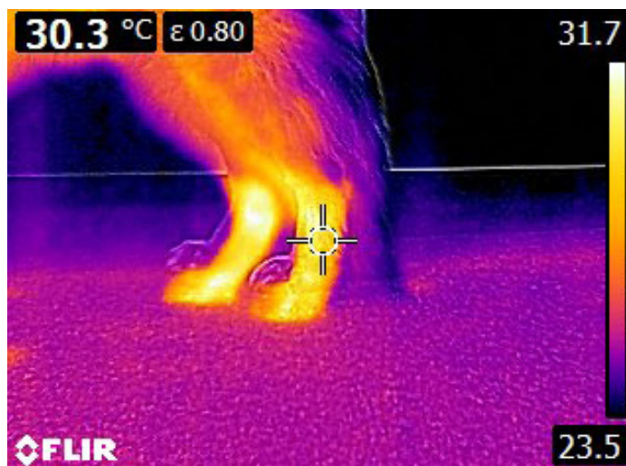
Fig. 5: Thermal imaging of the dog's skin temperature after 2 hours of wearing the orthosis featuring TPU lattice structures.
